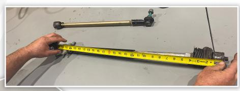
ONCE THE TIE ROD END AND THE INNER TIE ROD END ARE COMPLETED SET THE TIE ROD TO THE STOCK TIE RODS MEASUREMENT. NOW, USING AN ALLEN WRENCH SET THE FIRST SET SCREW ONCE IT IS ALIGNED ALONG THE CHANNEL ON THE TIE ROD AS SEEN IN THE IMAGE TO THE LEFT. NOW SET THE SECOND SET SCREW ON THE SIDE.
