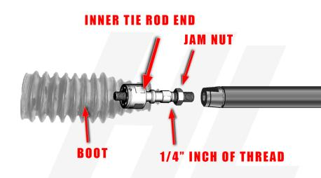
5. SET THE LENGTH OF THE NEW ADJUSTABLE TIE ROD TO THE MEASURED LENGTH OF THE ORIGINAL TIE ROD. DO THIS BY ADJUSTING THE TWO TIE ROD HALVES.
