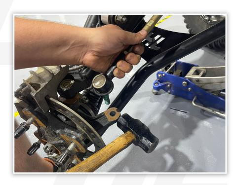
REMOVE CLAMPS AND/OR ANY ZIP TIES HOLDING THE BOOT IN PLACE. NOW, SLIDE THE BOOT DOWN THE TIE ROD.
