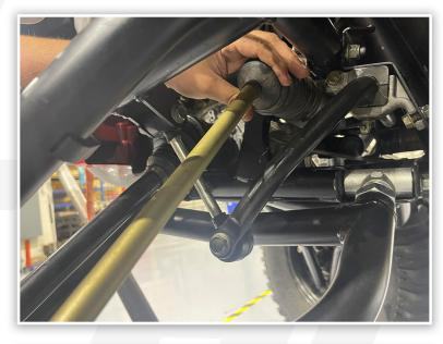
NEXT, LOOSEN THE INNER TIE ROD END FROM THE RACK.
