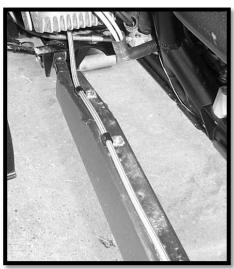
5. Disconnect the caliper/knuckle/hub assembly and radius bars from the factory trailing arms.
