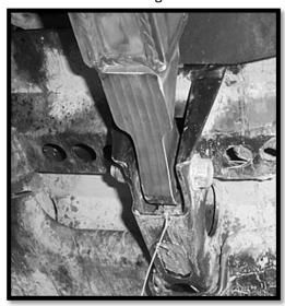
10. Connect the shock to the new trailing arm using the factory hardware.
