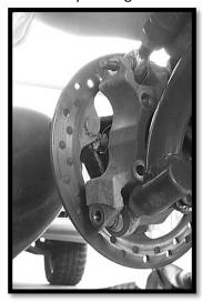
6. Next, disconnect the arm from the shock at the shock mount point. Remove the shock dust shield from the shock.
