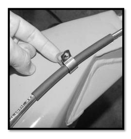
21. Make sure the brake line does not get pinched or cut during installation. There are predrilled holes in the arms to attach the remaining factory p-clips to using the **#12-1" Tek self-tapping screws**. Do not over torque.
