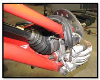
6. Disconnect the arm from the shock at the shock mount point.
