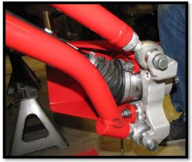
16. Install the rotor assembly and brake caliper using the factory hardware.
