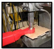
10. With the bearing seated all the way, you can now install the **100A** snap ring into the groove. If there's not enough room, you need to press the bearing in more.
