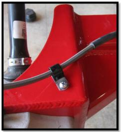
20. You will use your factory p-clamp next. The section of the brake line that has a strip of rubber surrounding it should line up with the next hole. <u>If it does</u>, you need to remove the piece of rubber that's inside your factory p-clamp and install the clip facing the correct direction as shown below. <u>If it doesn't</u>, then simply install it normally. Use a **#12-1" Tek self-tapping screw**. Do not over torque.
