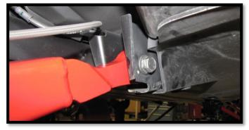
13. Connect the shock to the new trailing arm using the factory hardware. Make sure the brake line is to the <a href="outside">outside</a> of the shock tabs as shown below.
