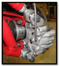
17. Attached the factory sway bar link to the new trailing arm using the factory hardware. Make sure the brake line runs <u>under</u> the sway bar link as shown below.
