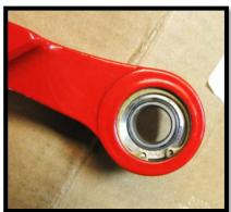
11. Insert a misalignment bushing 100F into both sides of the bearing.
