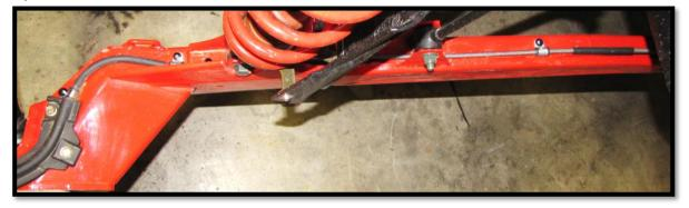
5. Disconnect the brake line guide/caliper/hub assembly/radius bars and knuckle from the factory trailing arms.
