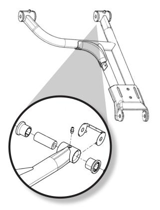
Remove the upper control arms at the frame by removing the frame bolts. (17mm) KEEP **FACTORY HARDWARE.**
