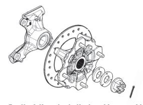
Reattach the rotor to the knuckle assembly. Install washers, then secure using the axle nut and cotter pin. (30mm)
