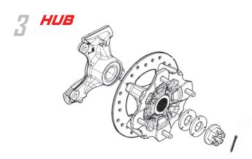
Remove the cotter pin, castle nut (30mm) and washers from the rear axles, then remove the brake rotor assembly.
