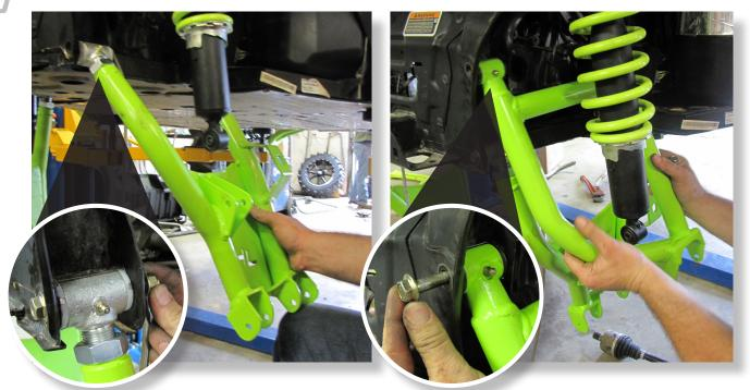
Install the new **LOWER control arm** to the frame, using the factory hardware. (17mm)
