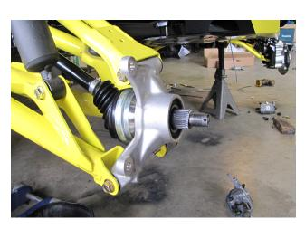
Remove the bolts and nuts that attach the rear knuckle to the upper & lower A-arms. (15mm) KEEP FACTORY HARDWARE.
