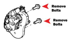
Remove the brake caliper mounting bolts from the hub assembly. (15mm) Set caliper aside. DO NOT DRAIN BRAKE FLUID.
