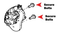
Secure the **brake caliper mounting bolts** from the hub assembly. (15mm) Set caliper aside.
