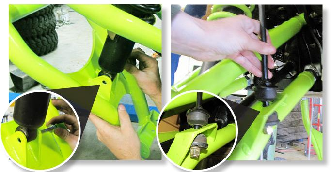
Secure the shock to the **LOWER** arm by installing a **M10x55mm bolt** followed by a **10mm washer** through the shock tab. Secure it with another **10mm washer** and **10mm lock nut.**
