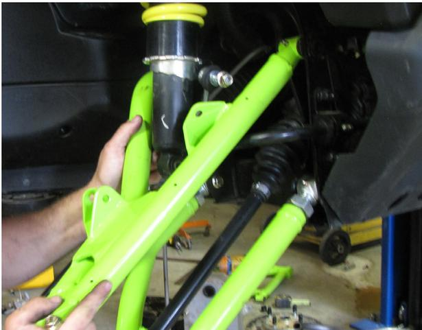
**Attach the new upper arm to the frame using factory hardware.**
