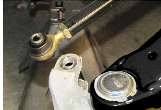
Remove the cotter pin, then remove the bolt and disconnect the tie rod end from the knuckle. (15mm) **KEEP ALL FACTORY HARDWARE.**
