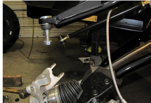
Disconnect the Upper arm by removing the cotter pin, then the bolts at the knuckle (19mm), sway bar, shock, and the frame. **KEEP ALL FACTORY HARDWARE.**
