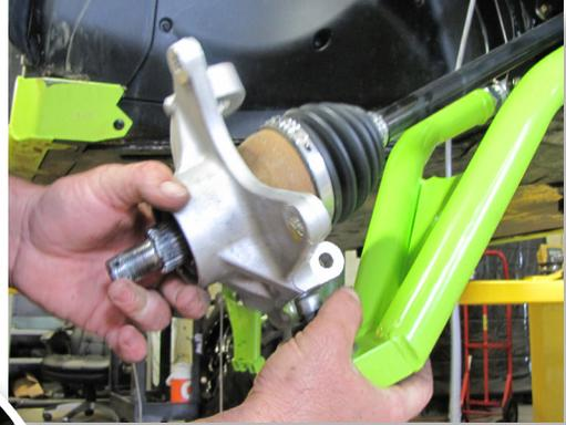
**Connect the hub at the LOWER pinch bolt FIRST, then slide the axle through AFTER. (19mm)**
