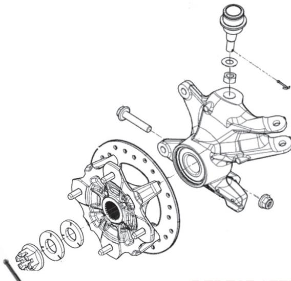
Remove the cotter pin, axle nut, and washers from the hub assembly, then remove the hub. (30mm)
