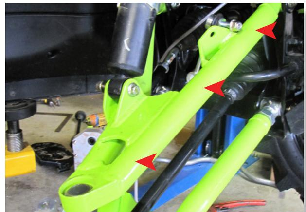
Route the brake lines down the FRONT of the upper control arm. Secure them with the 133B brake line clamps
