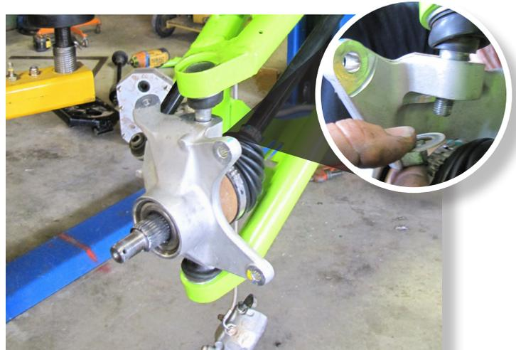
**Secure the upper arm at the knuckle using the factory washer and nut. Install the cotter pin.**
