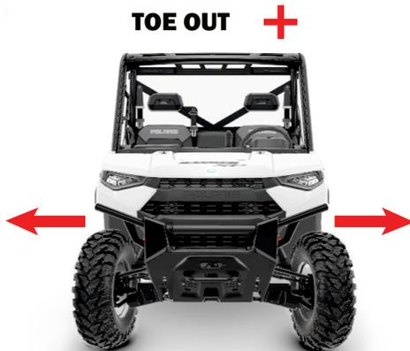
If the **FRONT OF THE WHEELS** are facing **OUT**, adjust the tie rods **OUT** or **INCREASE the length of the tie rod.**
