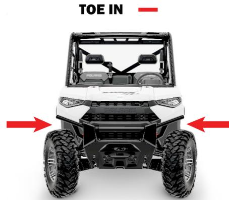
If the **FRONT OF THE WHEELS** are facing **IN**, adjust the tie rods **IN** or **REDUCE the length of the tie rod.**
