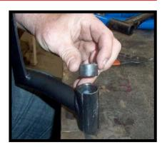
Reinstall the bushings, sleeves, and pivot caps into the new arm.
