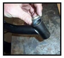
NOTE: Applying grease to the bushings and sleeves will make the installation easier.
