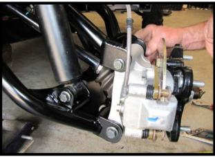
Attach the lower arm to the hub assembly using factory hardware. DO NOT FORGET WASHERS.
