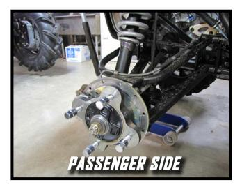
Place jack under the rear center of the UTV and lift until the weight is off the suspension. Ensure that the vehicle is properly secured, so that it is stable on the jack.
