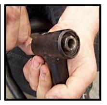
Use caution when removing the bushing from the collar, there is a stop built into the factory arm that prevents the bushing from pushing out when installed. Because of this, the bushing must be pushed out from the opposite side!! A flat punch or press is recommended to remove the bushings.
