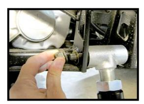
Connect the new lower arm to the frame using the factory hardware. **DO NOT FORGET WASHERS.**
