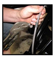
Drill out the factory p-clamps until they snap off, then remove the clamps.
