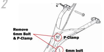
Disconnect brake lines by removing the 6mm bolt from the p-clamps from under the arm. DO NOT DISCONNECT BRAKE LINES FROM THE CALIPER.
