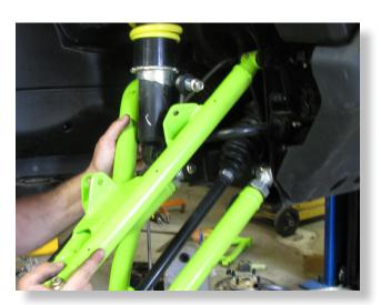
Attach the new upper arm to the frame using factory hardware.
