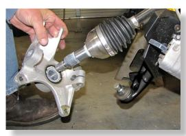
Remove the Lower Arm FIRST by removing the bolts at the knuckle (15mm) and the frame. KEEP ALL FACTORY HARDWARE.
