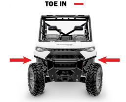
If the FRONT OF THE WHEELS are facing IN, adjust the tie rods IN or <u>REDUCE the length of the tie rod.</u>
