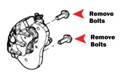
Remove the **brake caliper mounting** bolts from the hub (**15mm**) Set caliper aside.
