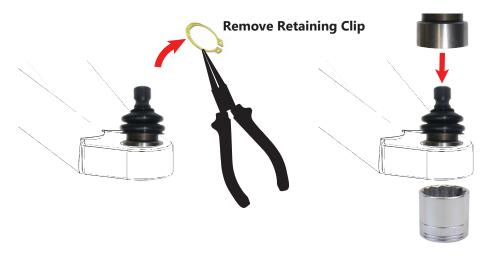
Back the ball joint with a large 36mm socket or something sturdy of similar diameter, then using a press or vice, press the ball joint out of the arm. BUSHINGS \_\_\_\_\_Install
