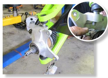
Secure the upper arm at the knuckle using the factory washer and nut. Install the cotter pin.
