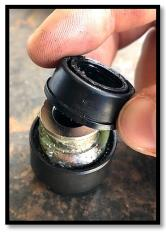
11. To press the joint in straight to the new trailing arm, first find a socket or pipe that fits just to the outer diameter edge of the joint.
