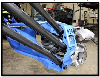
5. Disconnect the shock from the trailing arm.
