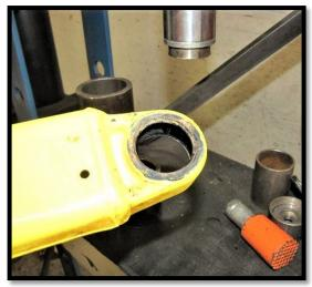
10. Before pressing the joint into the new trailing arm, we recommend removing a boot from one side to prevent any damage while pressing it in. Use a flat head, pinch with your thumb, and then pull it up.
