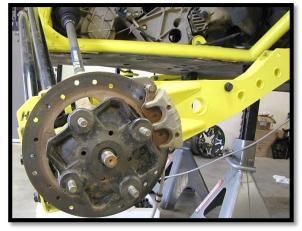
17. Attach the factory sway bar link to the new trailing arm using the factory hardware.
