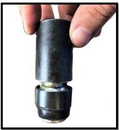
12. Find the new passenger side **trailing arm 120L-R**. Apply a small amount of grease to the joint, then place it <u>STRAIGHT</u> into the bracket. Use a press or vise to press it in <u>STRAIGHT</u> until it stops against the lip.
