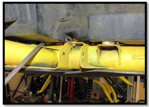
7. Next, you will need to remove the radial joint from the factory trailing arm. The factory radial joints will be re-used if they are in good condition.
