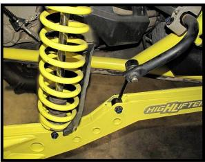
18. Attach the brake line to the predrilled holes on the back side of the trailing arm by using the factory p-clamps and the **#12-1" Tek self-tapping screws**. <u>Do not over torque.</u>
