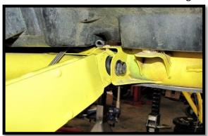
15. Connect the shock to the new trailing arm using the factory hardware.
