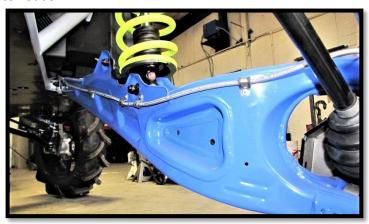
4. Disconnect the brake caliper/hub assembly/radius bars and knuckle from the factory trailing arms.
