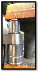
13. Once the retaining ring groove is visible, you can then re-install the boot. Use a flat head to press it back in and take care not to damage it. Then place and snap in the **retaining ring 112H**.
