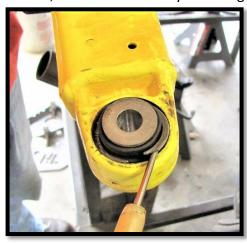
9. One side of the radial joint bracket has a lip, and the other side doesn't. Using a press or vise, you will need to CAREFULLY press the joint out of the bracket from the lipped side.
