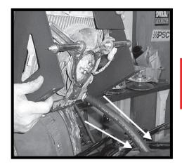
You need to insert the hose through the hole you drilled in the plastic as you are installing the radiator relocation kit to the rack.
