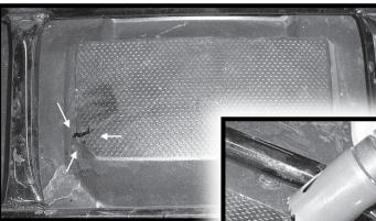
With a hole saw, drill the hole in the plastic, it needs to be 1 %" in diameter.
