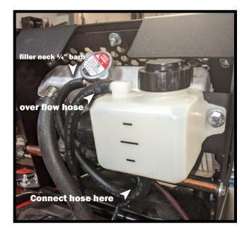
Connected to the radiator filler neck is a ¼" barb, cut 10" of the black ¼" hose provided, then connect the ¼" black hose to the barb on the filler neck and to the ¼" barb on the bottom of the over flow tank.
