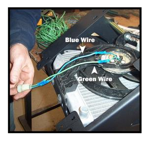
Using the **butt connecters** and **wire** provided, extend the **fan plug**. Attach the **green to green** and **blue to blue**.
