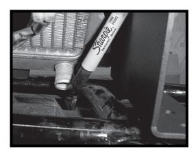
Mark all holes to be drilled for the radiator hose then remove the radiator from the rack.
