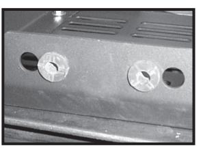
Where the bottom of the stock radiator attaches to the frame there are two **rubber grommets** that you will need to **remove** and place in the two center holes at the base of the new **face plate**.
