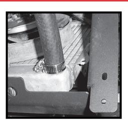
Connect 2ft of hose to the bottom of the radiator. Secure the hose to the lower portion of the radiator with the clamp provided.
