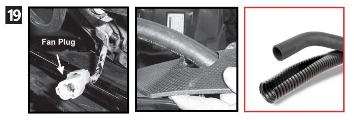
Push **the fan wire** through the **access panel** and reconnect it.
