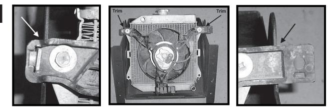
You will need to trim the stock radiator fan brackets, so that it will fit into the new shroud.
