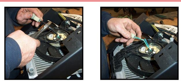
Cut the blue and green wire half way between the plug and the motor on the back of the fan.
