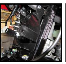
Bolt EPS mount to frame using 6mm x 16mm bolt, 6mm washer, and 6mm lock nut provided in the kit.
