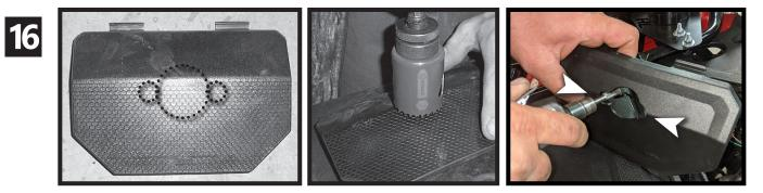
Locate the **access panel** and **cut** a **1**%" **in hole** in the center. If you **DO NOT have a rotary tool** we recommend you to use a **1/2 drill bit** to drill out holes on the side for extra wiring space **BEFORE** drilling the **1**% **hole**.
