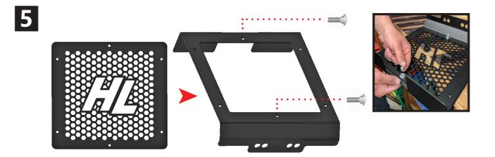
Start preassembling the the radiator mount by placing the **face plate BEHIND** the **plate frame** and install the **two 1/4 X 3/4 carriage bolts** to the center bolt holes then back it with the **two 1/4** washers and 1/4 lock nuts provided.
