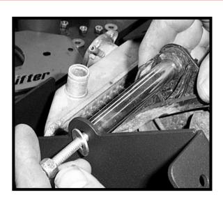
Next use the two **large spacers and 1/4 X 5 bolts** to connect the fan to the brackets.
