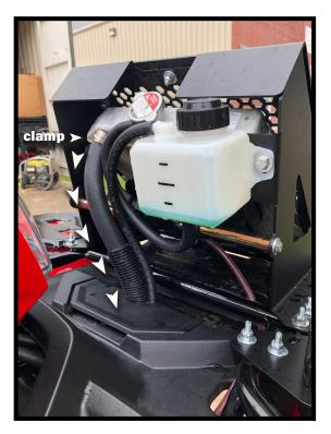
Route the hose through the access panel down, and leave hoses hanging below. Then connect the other end of hose to the top of the radiator with a clamp.
