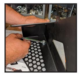
Attach the left and right leg, then begin installing the remainder of the carriage bolts washers and lock nuts and tighten them. (6 total)
