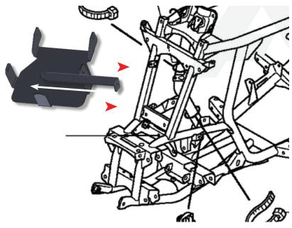
Once the **hoses** and **wires** are secure this will allow space for the **EPS unit** to be mounted to the frame where the **radiator** was previously mounted.
