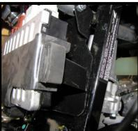
Locate the **EPS unit** and slide it over the prongs on the bracket.
