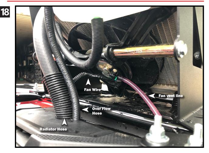
**IMPORTANT:** Place the **remaining loom** around the **hose** to keep it from rubbing on the rack and plastic fenders. If the hose is left unprotected the vibration of the hose against the rack and fenders will form a hole, causing fluid to leak out, potentially **RESULTING IN ENGINE DAMAGE. MAKE SURE ALL HOSES AND WIRES ARE COATED WITH LOOM.**
