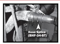
Once you have pushed the hoses through, connect the **inlet and outlet hoses** to the **hoses** you **left connect to the engine**. Secure the **hoses** to the **fitting** with the **clamps** provided in the kit.
