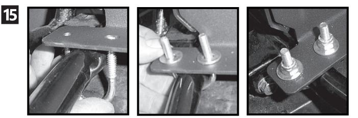
Connect the **radiator** to the **rack** using the <sup>1</sup>/<sub>4</sub> **x 1**" **bolts**, **U-bolts**, <sup>1</sup>/<sub>4</sub>" **washers** and <sup>1</sup>/<sub>4</sub>" **lock nuts** provided in the kit.
