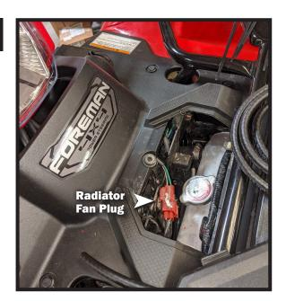
Remove the cover from the top of the ATV to access the radiator, then unplug the radiator fan plug.
