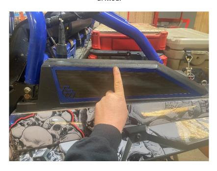
STEP 2: Using a 1/8" drill bit, drill the holes to mount cover.
