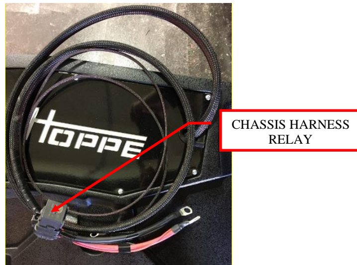
Figure 1: Chassis harness relay.
