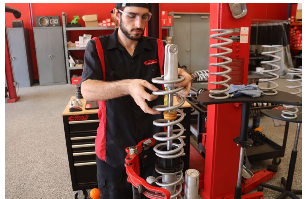
Install the Eibach main spring.
