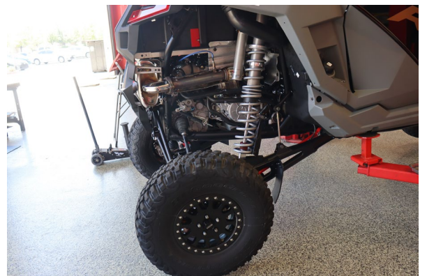
Reinstall the shock assembly and repeat on the opposite side. Torque shock bolts back to factory spec.
