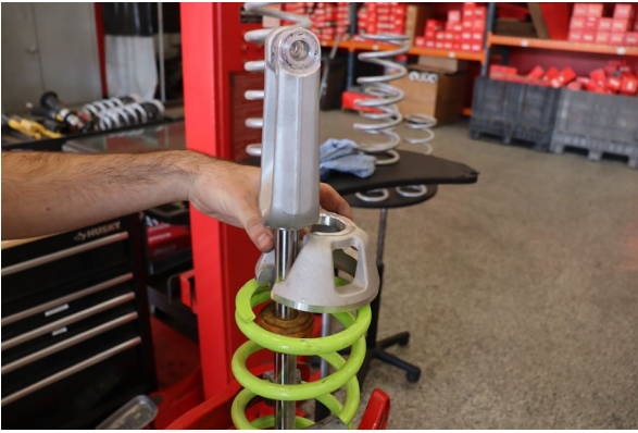
Compress the springs and remove the lower spring perch, OE springs, and slider.
