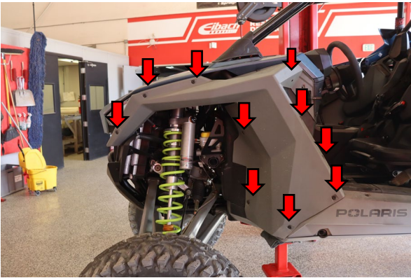
Remove the T40 torx bolts and clips on the fender and remove the fender.
