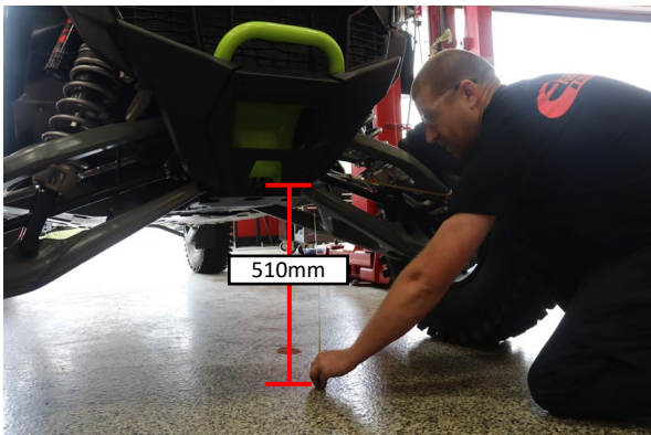
The front ride height should be about 510mm front the ground to the lower control arm bolt.
