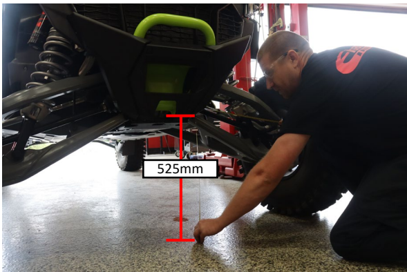
The front ride height should be about 525mm front the ground to the lower control arm bolt.
