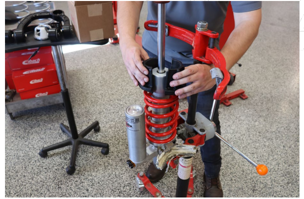
Remove the stock slider.
