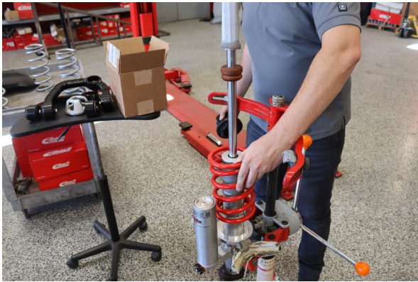
Remove the OE front tender spring.
