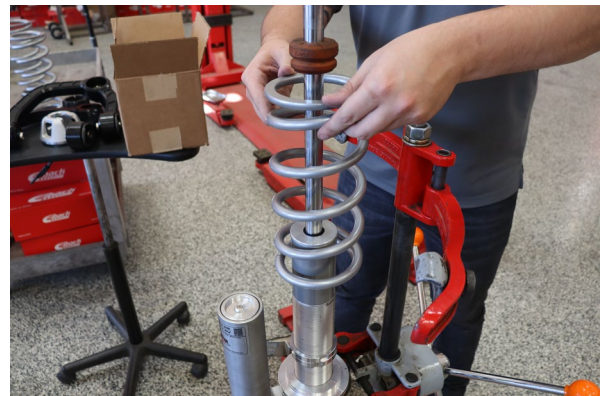
Install the Eibach Front Tender.
