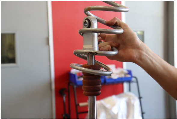
Install the Eibach rear tender spring.
