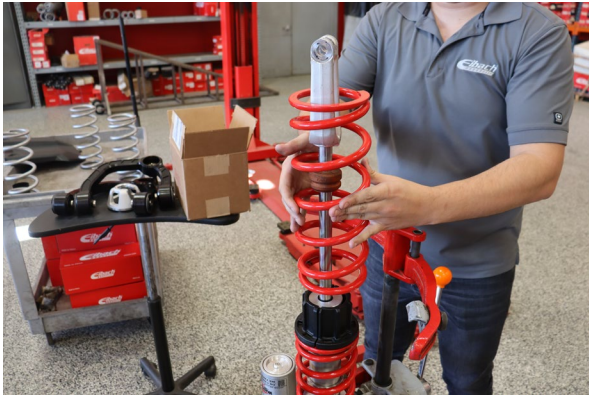
Remove the OE main spring.
