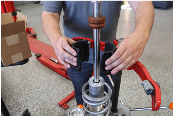
Install the OE 2-piece slider.
