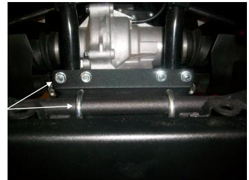
Use the 8mm bolts and washers on the underside of the mount and they will tread into the frame tubes. Tighten securely.
