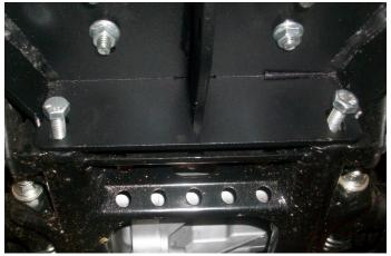
There are spacer provided for under the front location of the winch mount. These are needed for U-bolt clearance.
