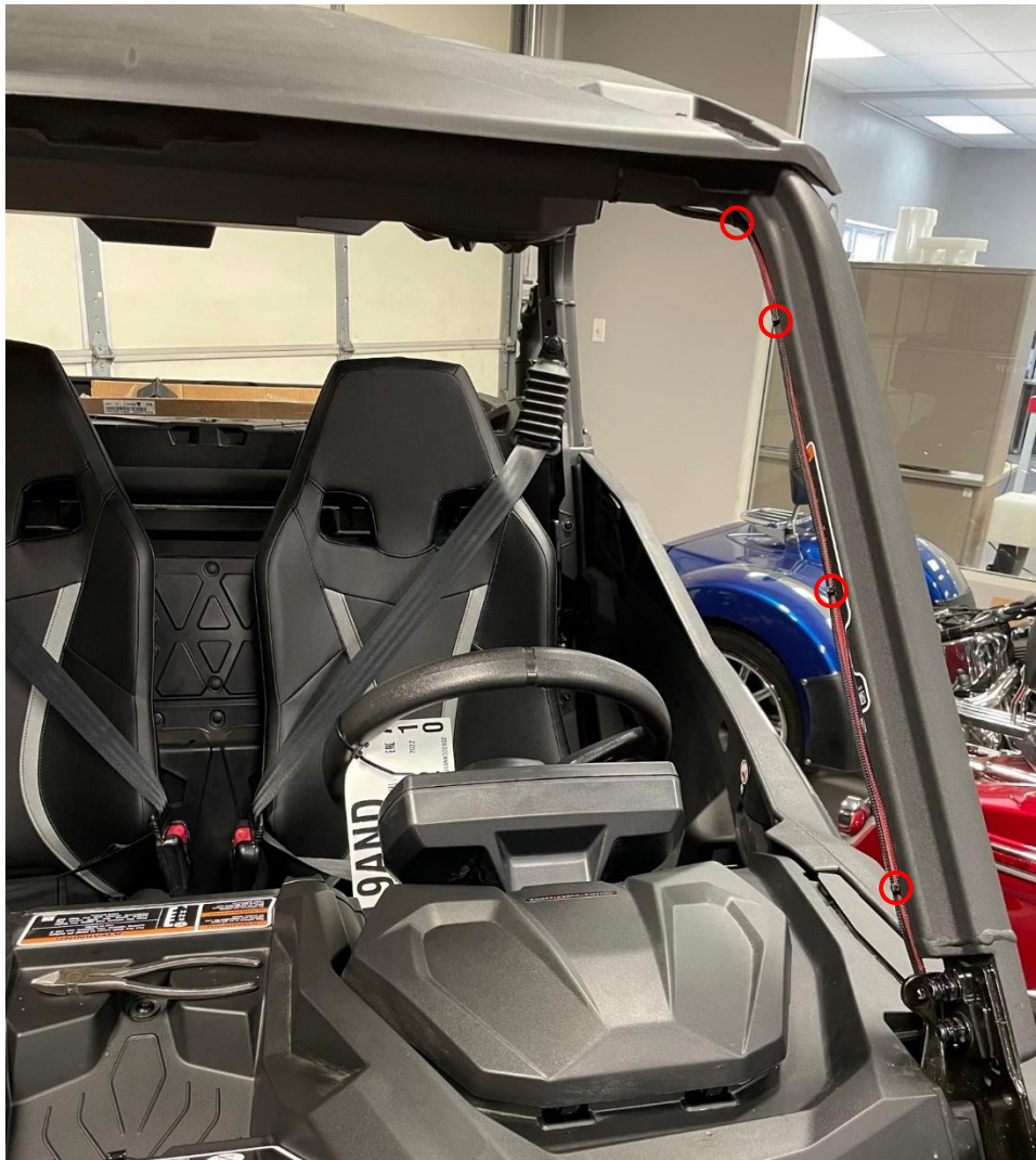
Figure 9: Route the chassis harness up the driver's front frame tube.
