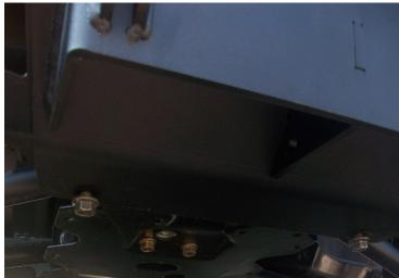
Get all 6 bolts in place and then tighten up firmly To make mount is secure. Attach push tube to tabs with pins included with push tube kit.
