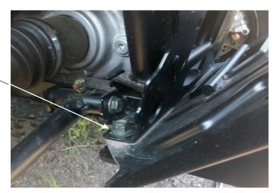
Mount plow mount up to the front of machine as shown using the  $4-7/16 \times 1$  hex bolt and nylock nuts on the upper portion of the mount. And re-use the bolts you took out at the bottom of the skid pan. Two of the 7/16 bolt are up under the push tube mount area.
