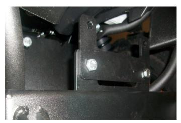
Push tube will mount with the wire loop pins that came with the push tube kit.
