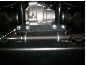
Use the 8mm bolts and washers on the underside of the mount and they will tread into the frame tubes. Tighten securely.
