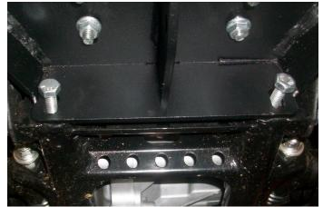
There are spacer provided for under the front location of the winch mount. These are needed for U-bolt clearance.
