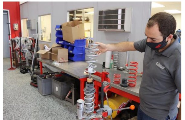
Step 12. Install the Eibach main spring (1000.300.0350S).
