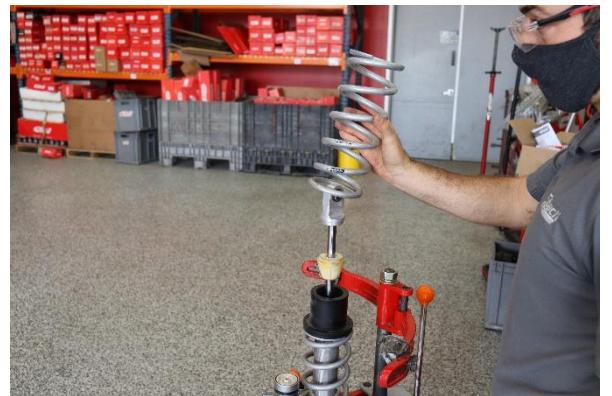
Step 12. Install the Eibach main spring (1000.300.0300S).
