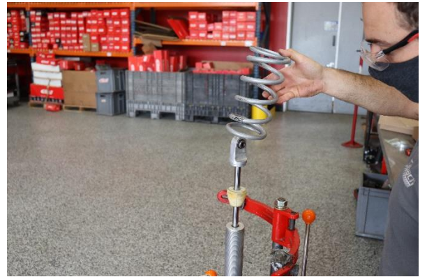
Step 10. Install the Eibach secondary spring (0800.300.0300S).
