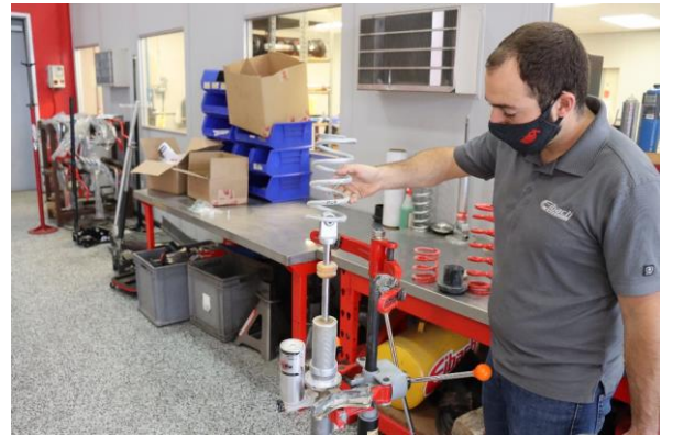
Step 10. Install the Eibach secondary spring (0800.300.0350S).
