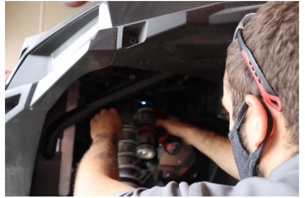
Step 14. Reinstall the coil over. Secure the coilover to the upper mount with the OE hardware.
