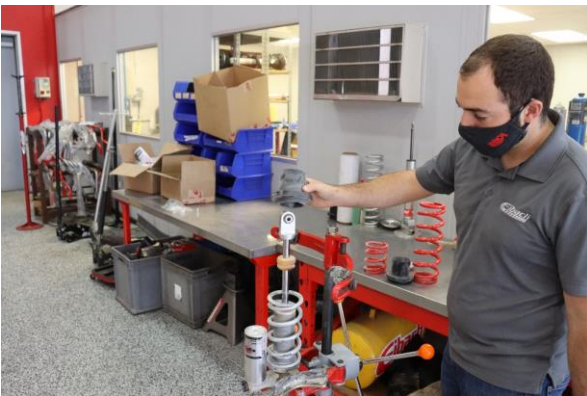
Step 11. Install the Eibach spring slider (8001064).
