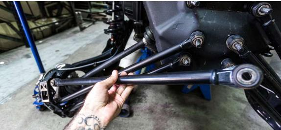
Step 5: Locate the correct size Agency Power Radius Rod for the top. Each of the rods are different size for top, middle and bottom. Use the corresponding OEM radius rod to adjust each Agency Power Radius Rods back to specification. Do this by matching up the agency power radius rod to the oem radius rod and inserting two bolts to match them up. Make sure the
