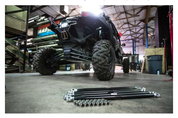
Step 1: Loosen the lug nuts on both rear wheels and lift the vehicle so that there is no tension on the rear of the suspension. Secure the vehicle with jack stands. NEVER attempt to work under any vehicle without properly securing it with jack stands. Please refer to your owners manual if you are unsure where to lift and support the vehicle.
