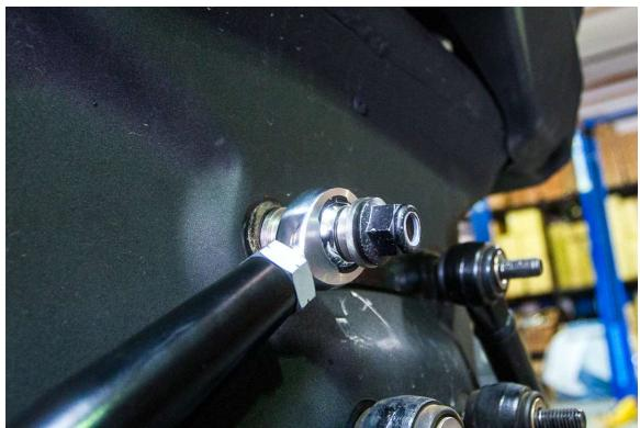
Step 7: Once all radius rods are installed. Remove the nuts from the chassis brace bolts and reinstall the chassis brace plate. Use red thread locker on all non-nylon hardware to prevent loosening and torque to OEM Specs. (Do not over-torque). After the first 50-100 miles recheck tightness of bolts to ensure appropriate torque spec
