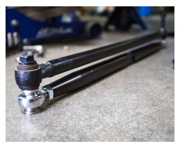
Step 6: Ensure that the stainless steel misalignment spacers are in place at each end of the heims and Insert the Agency Power Radius Rod into the hub and attach to the chassis brace bolt. Use the chassis brace nut to hold the radius rod in place while you continue to swap out the remaining radius rods. Continue the steps above for the remainder of the radius rods.
