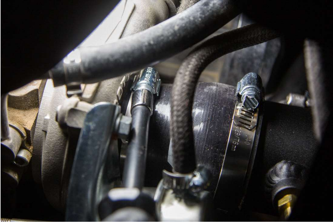
STEP 20 – Reinstall (boost solenoid) breather hose onto fitting.
