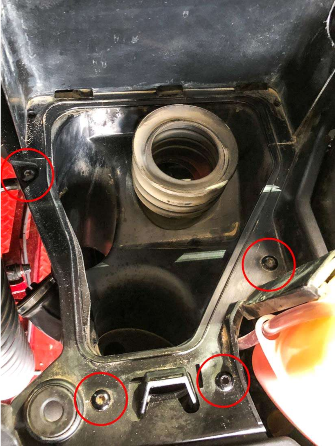
STEP 9 – Remove the indicated 4x T30 Torx Bolts around the top of the intake housing
