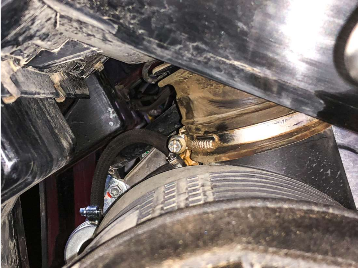
STEP 7 – Remove breather hose from intake boot and remove intake from vehicle
