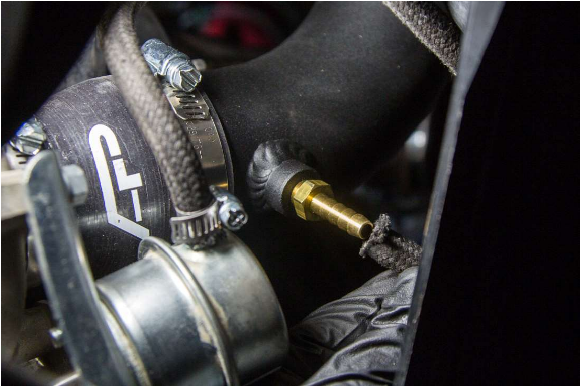
STEP 20 – Reinstall (boost solenoid) breather hose onto fitting.
