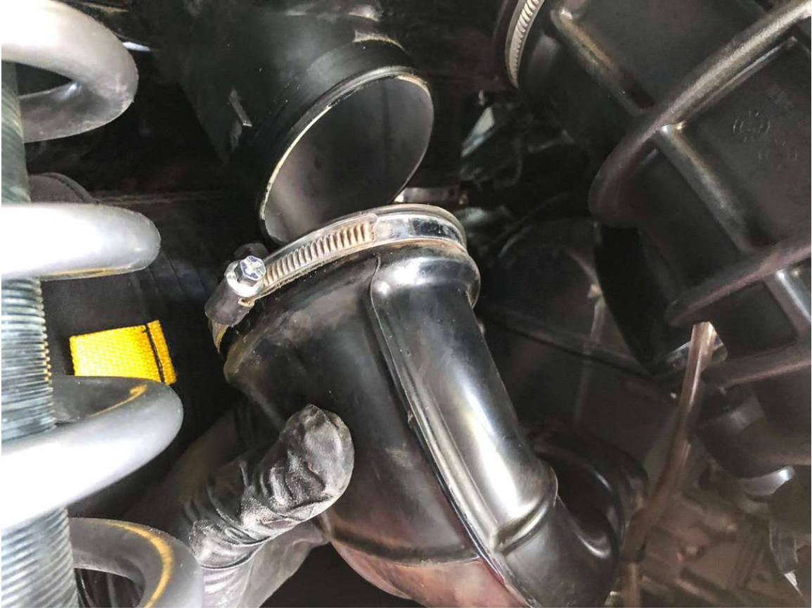
Loosen hose clamp on intake boot
