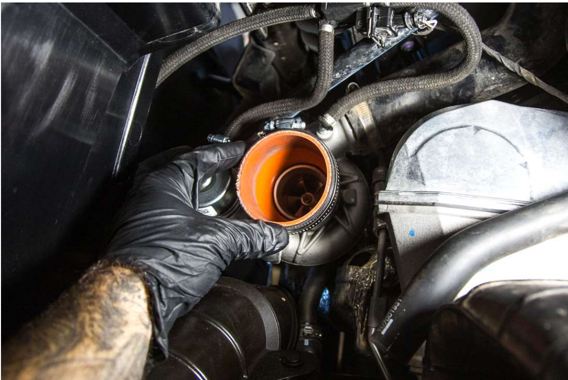
STEP 13 – Feed the new intake tube. For easiest install start with bracket and rotate intake
