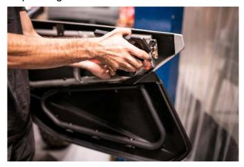
3) Next, we will want to clamp down on the rivet holding in the strap. The goal is to grab the rivet and stop it from moving, while leaving the center of the rivet exposed. This prevents the rivet from spinning when we drill it out.
