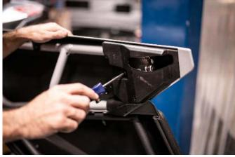
7) Attach the handle bracket to the latch arm. Use the 3mm hex key to secure the the remaining M5 screws.
