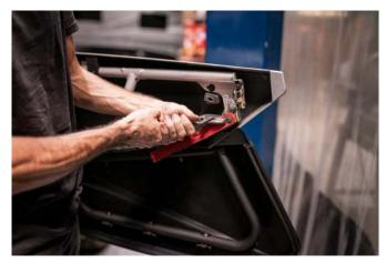
4) Drill out the factory rivet. **CAUTION:** Be careful to drill out ONLY the rivet. Do not widen the hole in the latch any wider. Doing so may cause play in the handle and may cause the latch to not work as intended.
