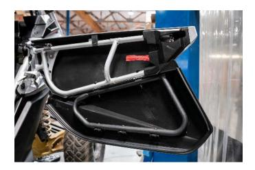
2) Remove the plastic cover which covers the latch. Remove the T30 screw in the center (NOTE: The X3 Max will have three 8mm screws in in the rear doors) and pry gently from the strap side. Thread the strap through the cover and remove the cover and set it aside.
