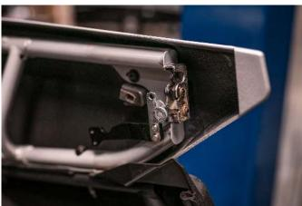
6) Reinstall the factory plastic cover. Thread the latch arm through the cover and snap it back into place. Secure the cover with the factory screw.
