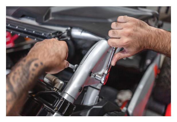
2) With the two nuts removed, place the Agency Power whip light mounting bracket on the two protruding cage bolts
