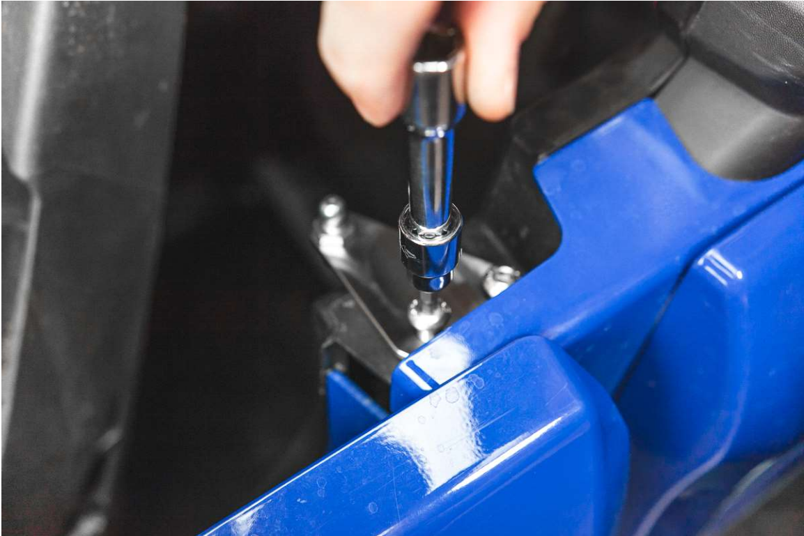
Step 5: Tighten both door hinge bolts with the HW5 bit and provided hardware.
