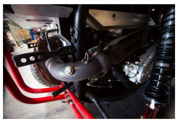
Step 7: With the exhaust out of the way you can now access the two bolts. Use a pry bar to support the engine and remove the hardware. Please note: The vehicle used in the this install guide had an aftermarket intake manifold and additional steps may be needed to remove the motor mount from the rzr.
