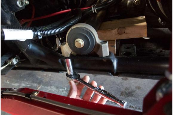
Step 2: Next support the engine mount bar by using couple small wood blocks or a pry bar.
