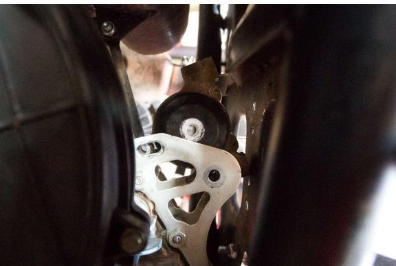
Step 8: Insert the new Agency Power Motor/trans Mount into place, re-use the hardware from the factory motor mount. If needed use a pry bar to align the bolt holes of both the motor
