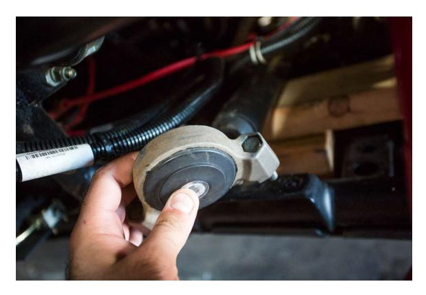
Step 3: Remove the two bolts from the factory motor mount. These are held in with a small retaining clip and can be tapped out. This retaining clip will no longer be needed for reinstallation.
