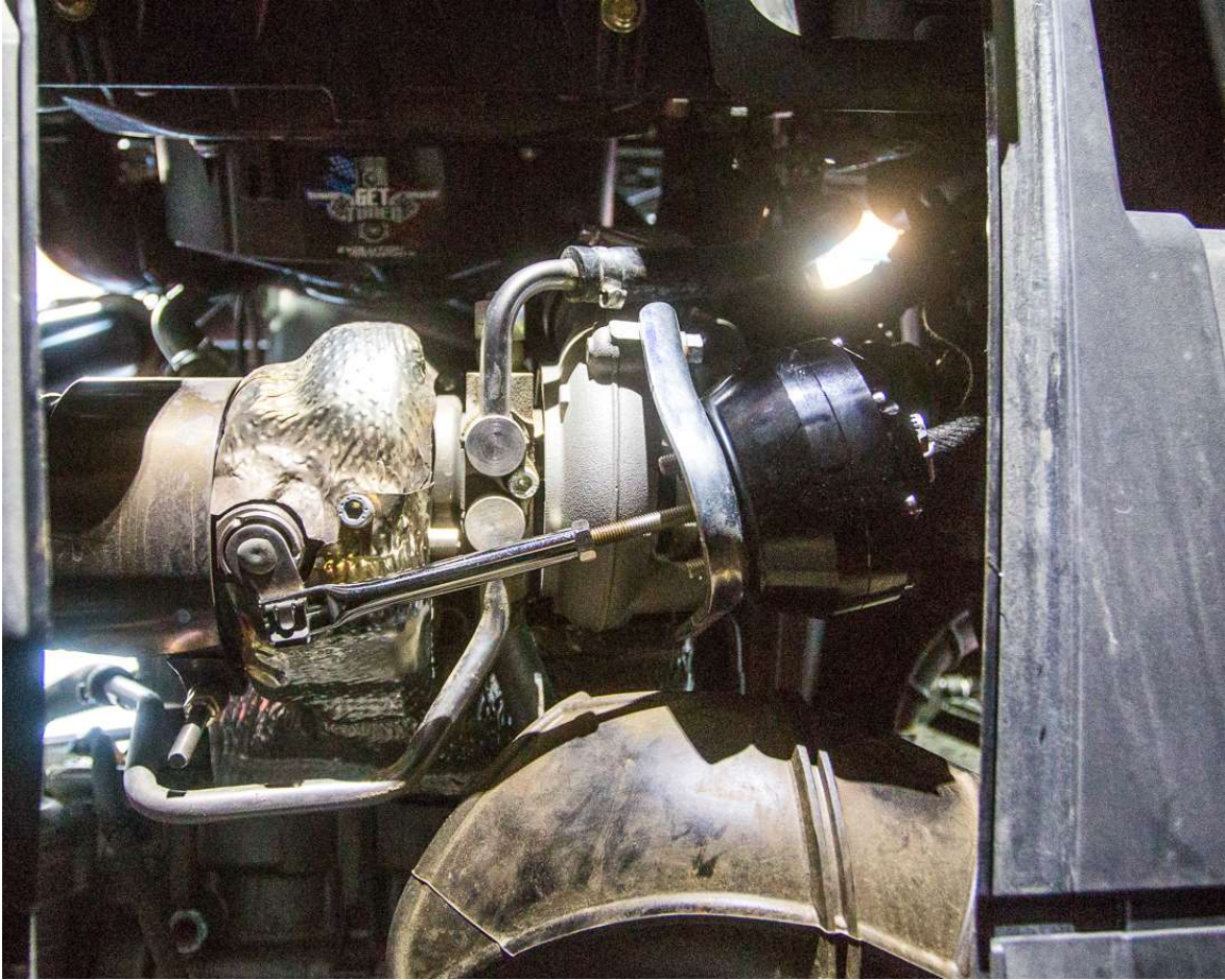
FINISHED – Congratulation on installing the Agency Power Wastegate for the Can-Am Maverick X3
