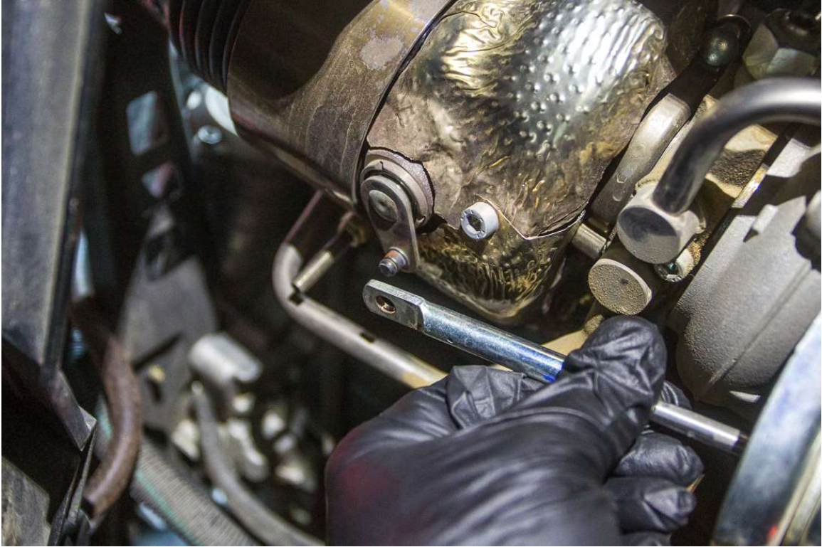
Step 2 – Remove the 10mm nuts holding on the stock wastegate.
