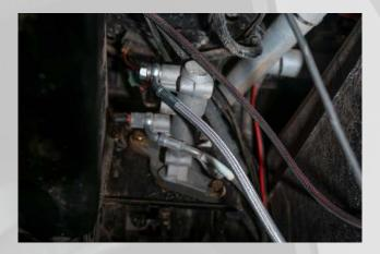
12. Route the brake line beneath the dash and to the other side. Route the brake line under the center console for the most clearance. Connect the line to the handbrake master cylinder, farthest port from the bracket using the 7/16-20 x 24mm banjo bolt. Connect the factory brake line to the second port, closest to the bracket using the 3/8-24 x 20mm banjo bolt.
