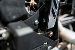
10. Mark where the handbrake base meets the console. Remove the handbrake and carefully drill 1/4" holes into the center console.
