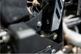
14. Install the M6 x 25mm bolts, small M6 washers, and M6 Nyloc nuts through the newly drilled lower mounting holes.
