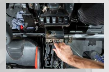
6. Relocate the power distribution block and clip towards the rear of the vehicle.
