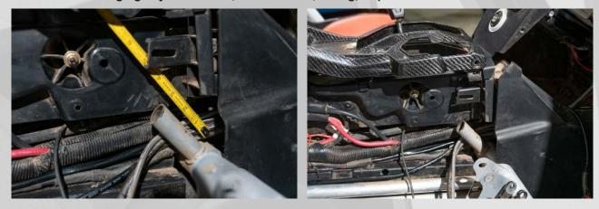
8. Trim the interior plastic tab as shown and tuck the wiring harness below the remaining piece of the grab handle tube.
