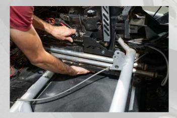
15.Recommended for additional stability: Drill a 1/4" hole through the factory grab bar tune and Agency Power front handbrake mount. Insert the M6 x 35mm bolt through the hole and secure with an M6 washer and Nyloc nut.
