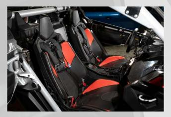
2. Unbolt the front of the seat from the support. Remove the seat bottom to gain access to the rear bolts. Unbolt the rear from the rear bulkhead.
