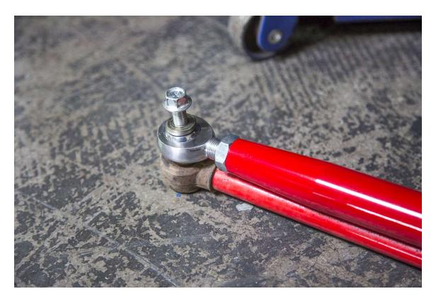
Step 5) Insert the misalignment into each end of the heim. The Heim attaching to the wheel hub assembly use the shorter misalignment spacers and the heims attaching to the radius rod plate (center of rzr) use the taller misalignment spacers.
