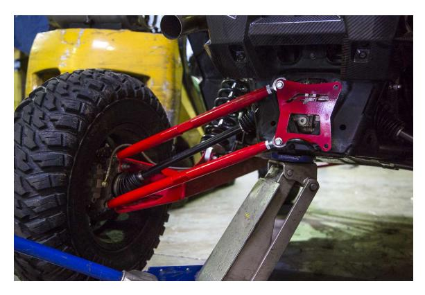
Step 7) Once the Radius Rods are installed, all of the hardware including the jam nuts can be tightened.
