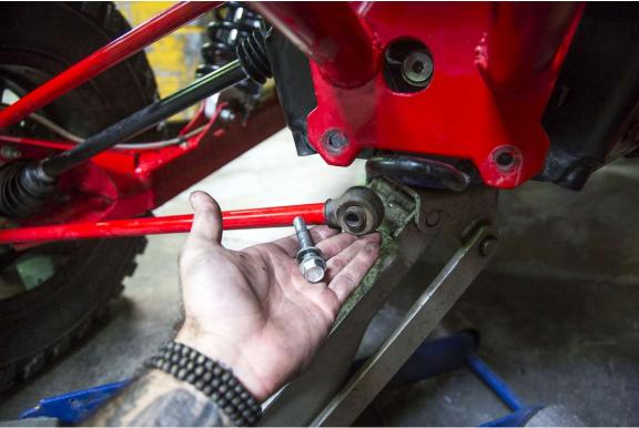
Step 3) Next remove the four bolts securing the radius rods to the rear wheel hub. Remove the
