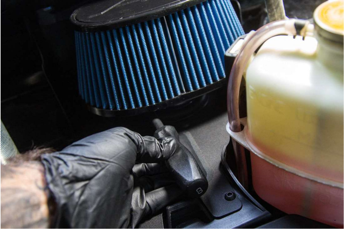
STEP 19 – Tighten clamps on turbo and intake tube.
