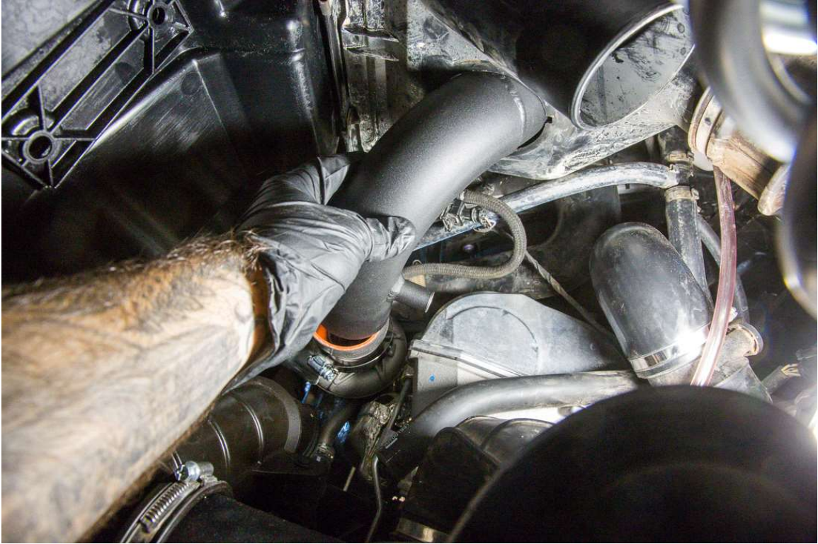
STEP 14 – Connect intake tube to turbo coupler.
