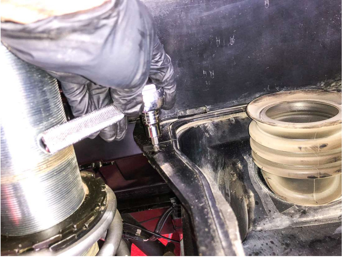
STEP 10 – Remove rubber tube from the intake housing.
