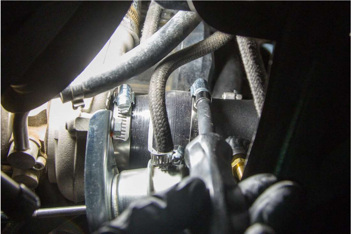
STEP 19 – Tighten clamps on turbo and intake tube.
