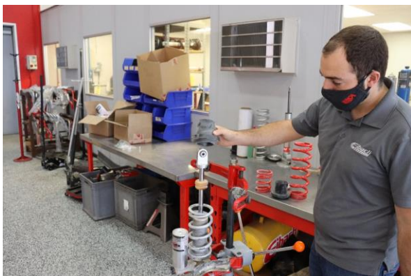
Step 11. Install the Eibach spring slider (8001064).
