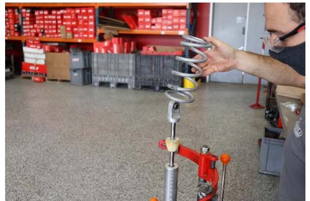
Step 10. Install the Eibach secondary spring (0800.300.0300S).
