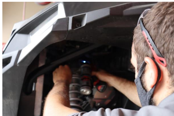
Step 14. Reinstall the coil over. Secure the coilover to the upper mount with the OE hardware.
