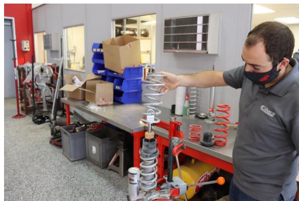
Step 12. Install the Eibach main spring (1000.300.0350S).
