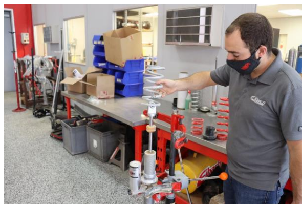
Step 10. Install the Eibach secondary spring (0800.300.0350S).
