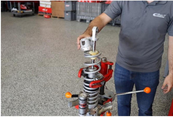
Step 13. Compress the spring assembly and re-install the spring retainer.
