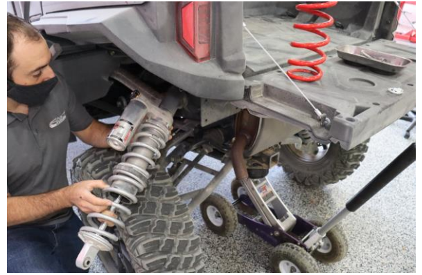
Step 14. Reinstall the coil over.
