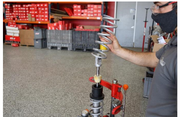
Step 12. Install the Eibach main spring (1000.300.0300S).
