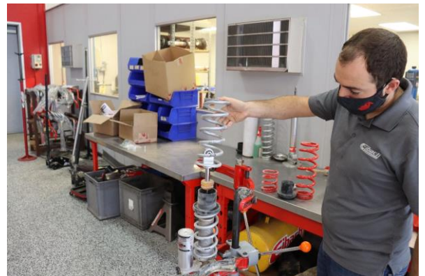
Step 12. Install the Eibach main spring (1000.300.0300S).
