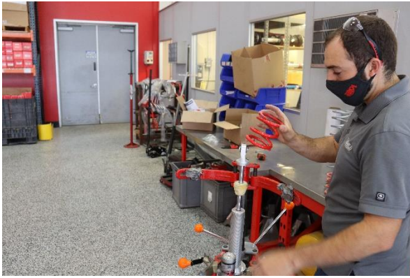
Step 7. Remove OE secondary spring.
