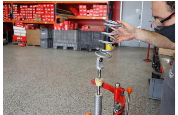
Step 10. Install the Eibach secondary spring (0800.300.0300S).
