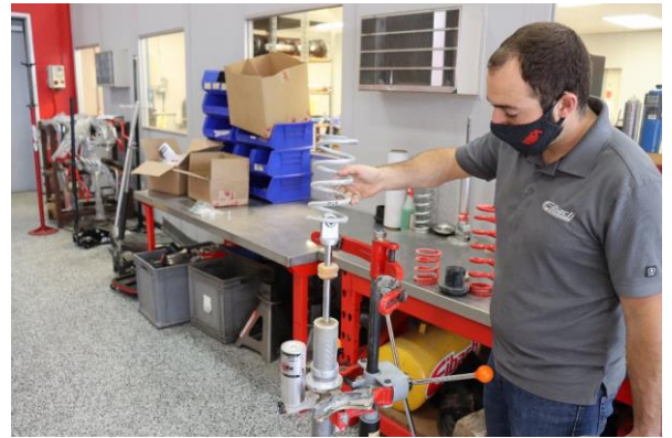
Step 10. Install the Eibach secondary spring (0800.300.0350S).
