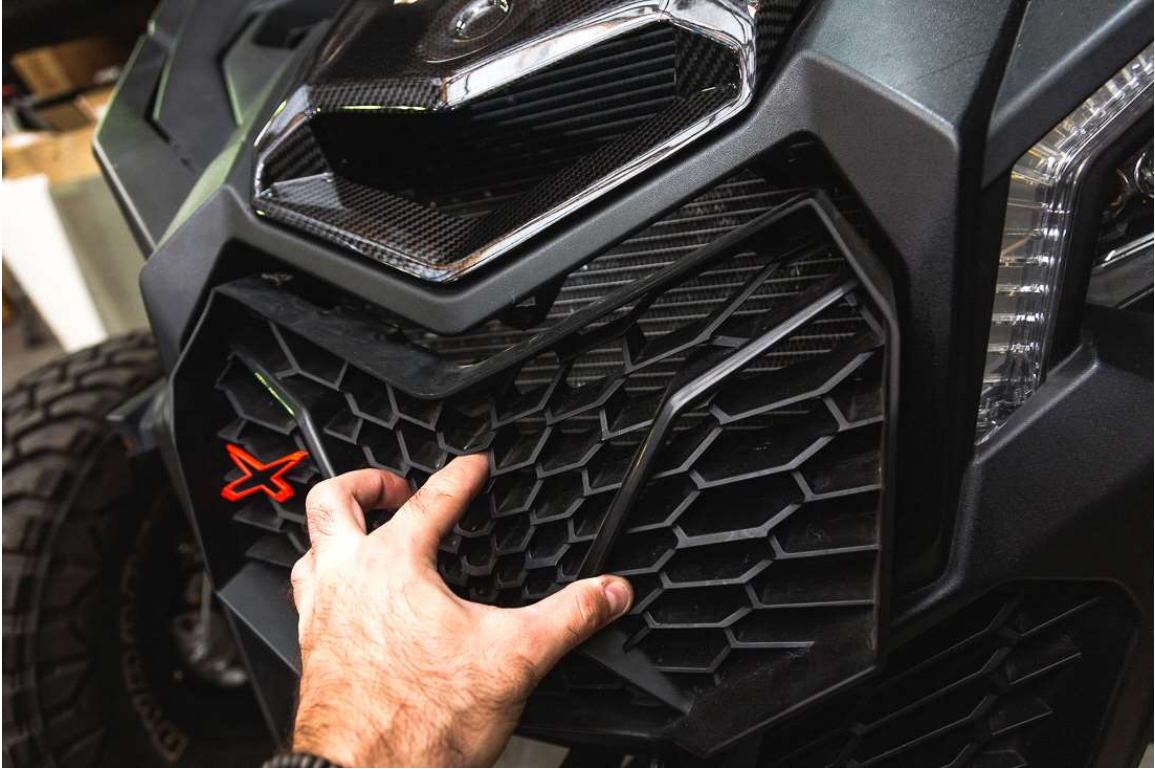
Close up look at the push clips that hold the factory grille in place.
