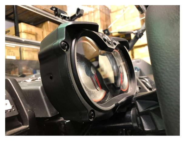
Step 1: Remove the 4x torx screws from the dash bezel
