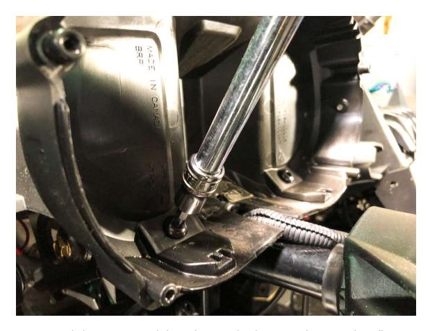
Step 4: Attach the new gauge pod plate in between the plastic gauge housing and install using the hardware that was removed on step 3
