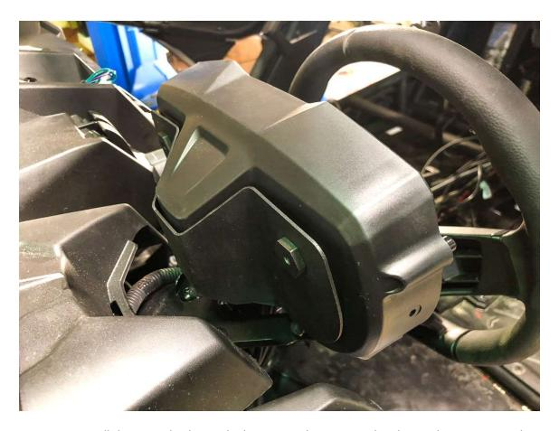
Step 5: Re-Install the gauge back into the housing and reconnect the electrical connector to the factory gauge.
