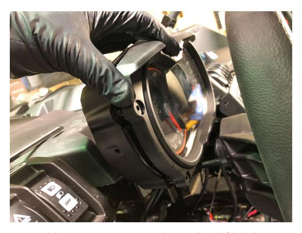
Step 6: Attach the Agency Power Hex Key Gauge Pod Mount to the back of the bracket using the provide hardware. Rotate the mount either counter or clockwise to desired position.
