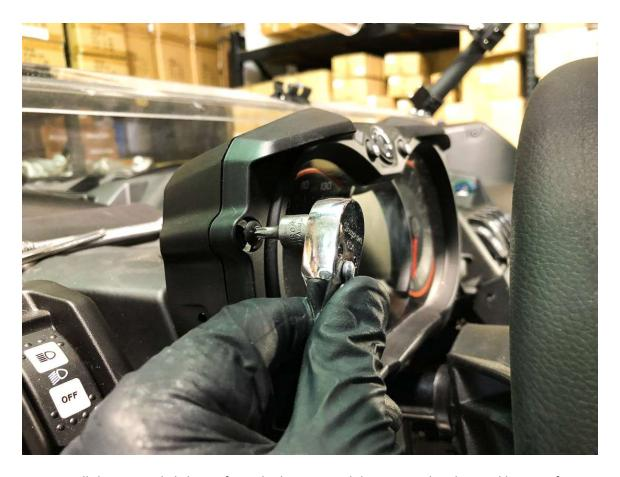
Step 2: Pull the gauge slightly out from the housing and disconnect the electrical harness from the back of the gauge.
