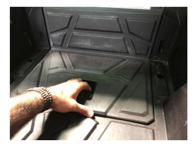
Step 2: Remove the factory ball style latch and replace with the provided push button latching mechanism. You will need to use a wrench on the underside of the latch to stop it from spinning. We recommend applying a small amount of Loctite to the threads when assembling the new latch.
