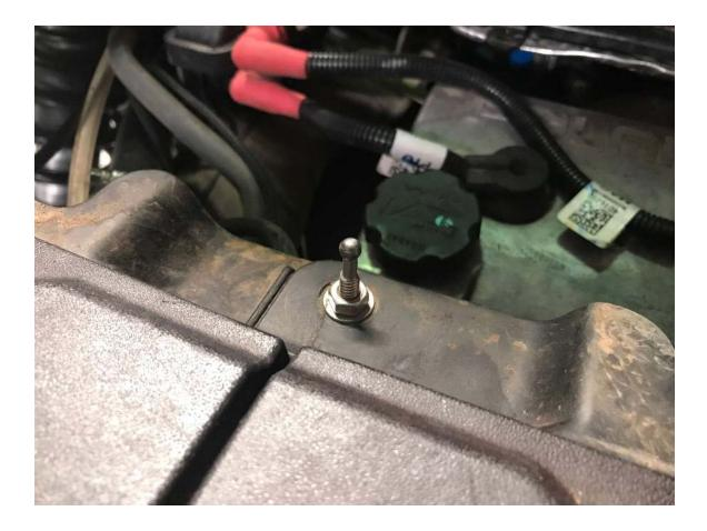
Step 3: Test fit the cover by inserting the engine cove into the upper tabs. If the cover fails to latch, remove cover and adjust the height of the ball latching bolt and refit cover until it securely latches to the engine cover.
