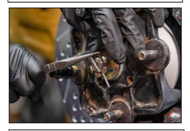
7. Install the cotter pin and bend one side on top of the axle end. Bend the other side down and away towards the hub face.
