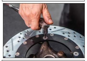
3. Using a 5mm allen head socket, tighten the bolts by hand. Tighten in a cross sequence to ensure the hat is flat to the hub. Once done torque these bolts to 25ft lbs.
