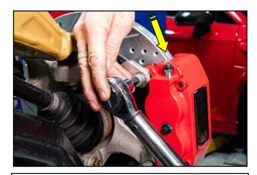
9. Verify there is not any rotor to caliper interference. (See arrow) Once verified torque these bolt to 58ft lbs.
