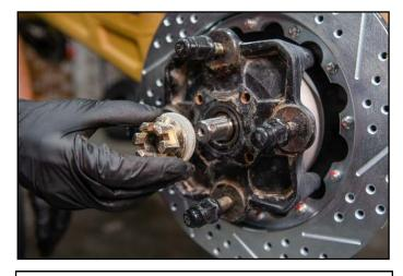
5. Install the factory washer (domed portion outward) and spindle nut onto the axle end. Select the 4WD position and place the transmission lever on 'P'. Using a 30mm socket hand tighten the nut to pull the axle fully through the hub.
