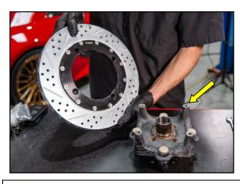
1. Start by inspecting the 4 mounting bosses on the hub and making sure they are clear of rust, debris, etc. Place the correct side rotor (Driver front shown) onto the hub and line up the 4 holes.
