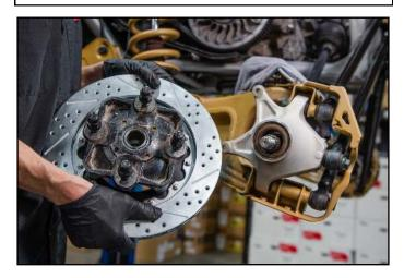
4. Next install the rotor/hub assembly onto the spindle by inserting the axle onto the splined portion of the hub. Now is a good time to inspect the outer seal, and replace if needed. Apply synthetic grease (XPS 293550010 or equivalent) around the drive shaft & splines. Be careful not to damage the outer bearing seal while installing the hub snout into the bearing. (Front Driver shown)
