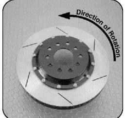
Non-modified or plain rotors that employ a curved vane design <u>must also</u> rotate in a specific direction. The curved vane rotor is designed to draw air into the center of the rotor and force the air to exit from the outer edge (see diagram on left).
