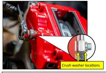
12. Make sure the banjo end is orientated as shown. Torque the banjo bolt to 12-15ft lbs.
