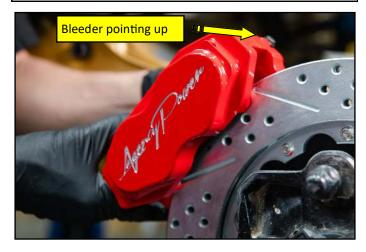
8. Next install the correct side caliper with the bleeder pointing up. Make sure the spindles caliper mounts are free from debris to ensure the caliper will sit flat. Use the supplied M10 x 30 SHCS bolts and tighten the 2 bolts by hand.
