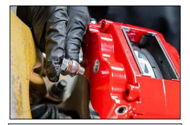
11. Using the supplied banjo bolts and crush washers install the factory hose to the caliper. Make sure you install one crush washer on each side of the banjo end of the hose.
