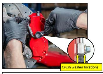
12. Make sure the banjo end is orientated as shown. Torque the banjo bolt to 12-15ft lbs.
