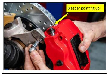
8. Next install the correct side caliper with the bleeder pointing up. Make sure the spindles caliper mounts are free from debris to ensure the caliper will sit flat. Use the supplied M10 x 30 SHCS bolts and tighten the 2 bolts by hand.
