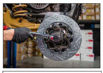
6. Once hand tight, torque this nut to 185ft lbs. Tighten the castle nut further slightly if needed to align the cotter pin hole.
