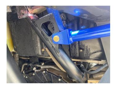
STEP 2: Install the shorter bolts into the lower frame. Use a washer on both sides.
