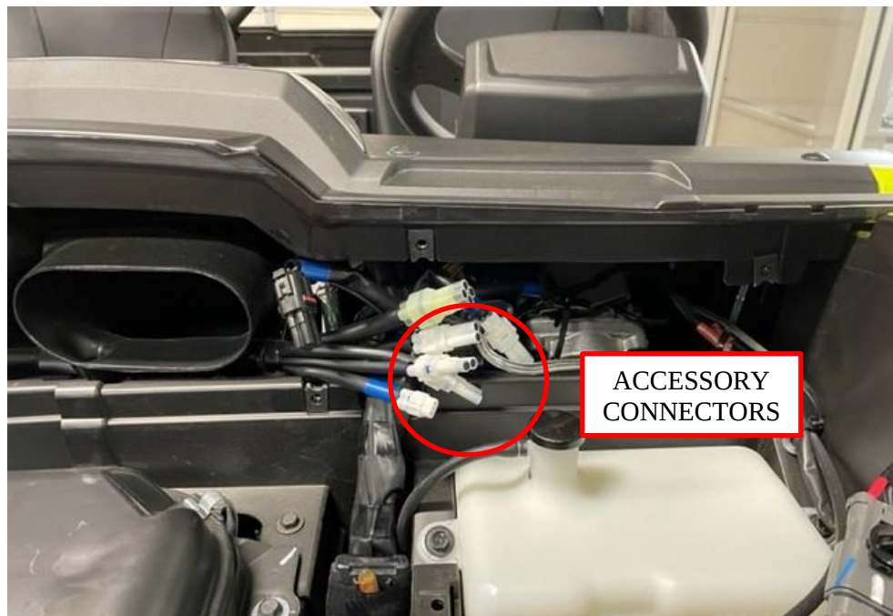
Figure 13: Accessory connectors for ignition power source.
