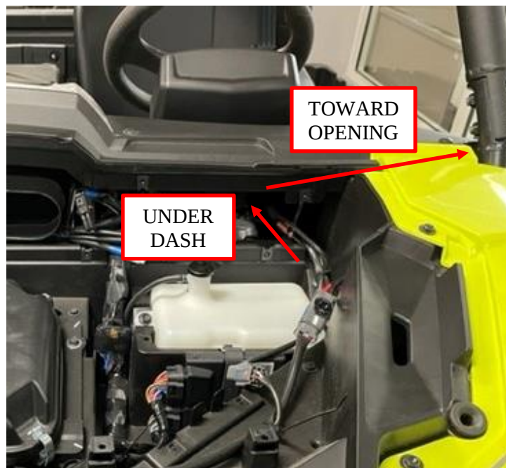
Figure 11: Chassis harness routing under dash to opening.
