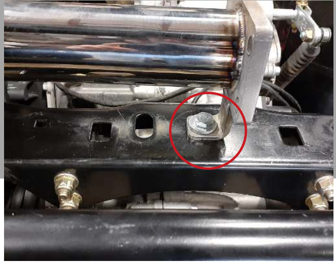
8. Set turbo assembly into chassis. Bolt down turbo assembly into vehicle. Tighten exhaust clamp and reinstall exhaust heat shielding. Reinstall stock O2 sensor and plug in
