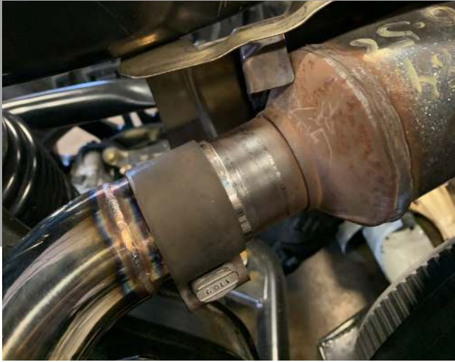
7. Install exhaust clamp onto turbo inlet pipe
