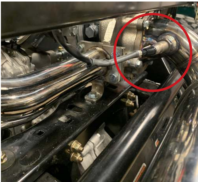
23. Install Dynojet AFR sensor into turbo exhaust. Run wires along right side of vehicle into the front cab area of the machine. Take care not to pinch or install the wire where damage can occur. Plug color matched wires into AFR Module
