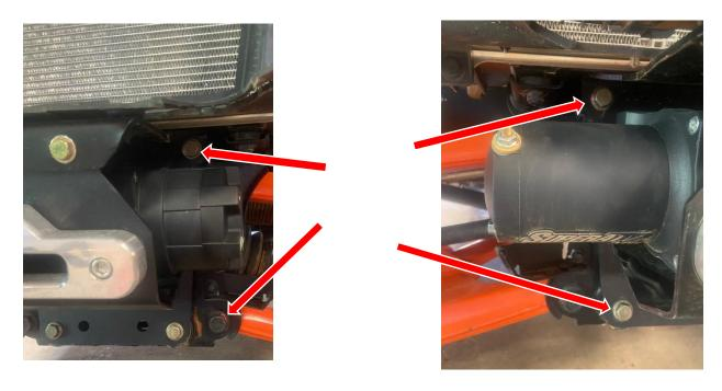
STEP 9: Install the factory push pins through the plastic and into the new winch plate.
