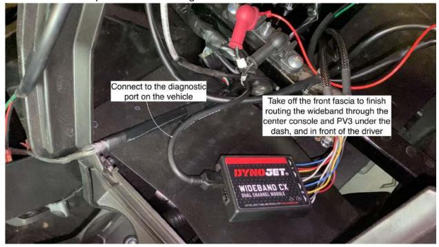
Route wideband under the dash and connect to the diagnostic port under the driver side dash.
