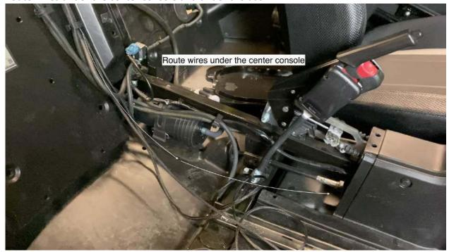
Take off the control panel to finish routing the wideband and PV3.
