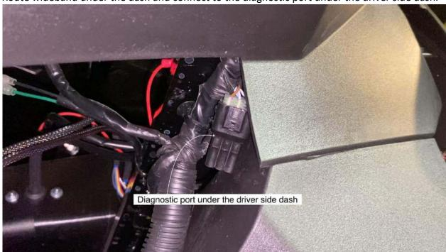
Route the PV3 wiring through the dash and mount where it is visible for the driver.
