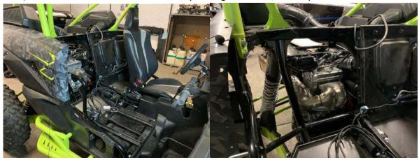
Remove exhaust muffler, header/mid-pipe from engine and EGT sensor, air intake tube, and the lower clutch air ducting tube.
