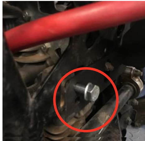
17. Install provided mounting bolts to bottom bracket through stock rubber mounts & bolt on the back side.
