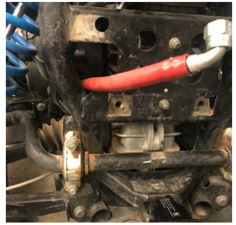
13. Install new oil drain line and route to back, making sure that it doesn't hit drive line.
