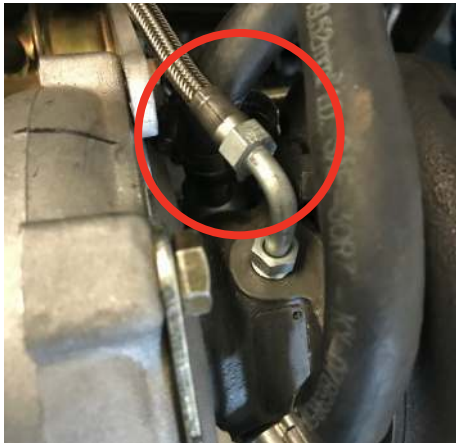
18. Install oil line to the turbo.
