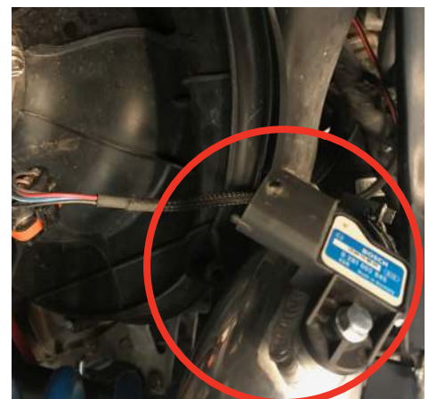
21. Install map sensor from Power Commander. IF YOU UPGRADED TO A POWER VISION, YOU DON'T NEED TO DO THIS.
