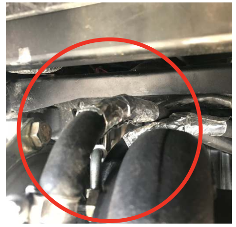
15. Install coolant lines to it BEFORE you mount the turbo assembly and wrap them with heat tape provided.
