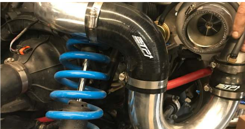
20. Install charge tube.
