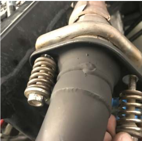
16. Now install bolts to exhaust.
