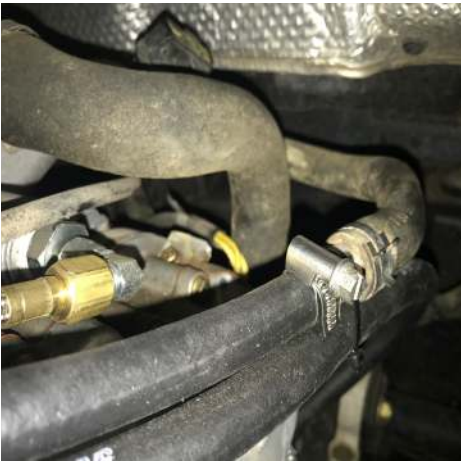
8. Install coolant line with coupler into stock hose that was take off from water pump.
