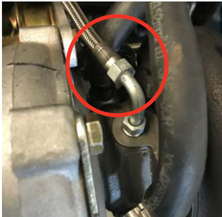
18. Install oil line to the turbo.
