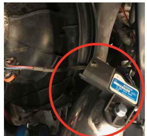
21. Install map sensor from Power Commander. IF YOU UPGRADED TO A POWER VISION, YOU DON'T NEED TO DO THIS.
