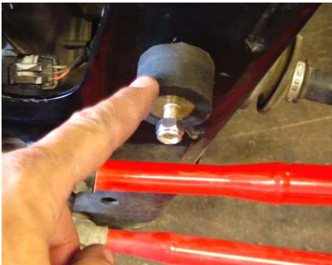
9. Drill out frame holes on the lower frame to 3/8", making them ready to accept rubber mounts
