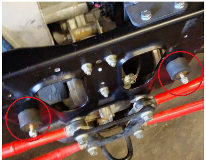
10. Install the rubber mounts that come attached to the turbo into the 3/8" holes that were just drilled in the frame. This is where the turbo will mount
