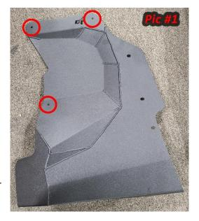
Install the T30 bolts into each of the 1/4" holes in your fender armor panel, loosely start a well nut on the back side of the bolt protruding through the panel. \*Pic #2
