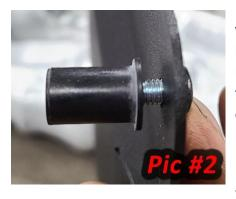
Install the panel by lining up the well nuts into the 1/2" holes you drilled out on the body. Install all remaining hardware loosely. Once the panel is in place and lined up with all hardware loosely installed, begin tightening the well nuts first (do NOT overtighten – if well nuts spin, apply pressure on panel to allow them to grab). Tighten all remaining hardware.
