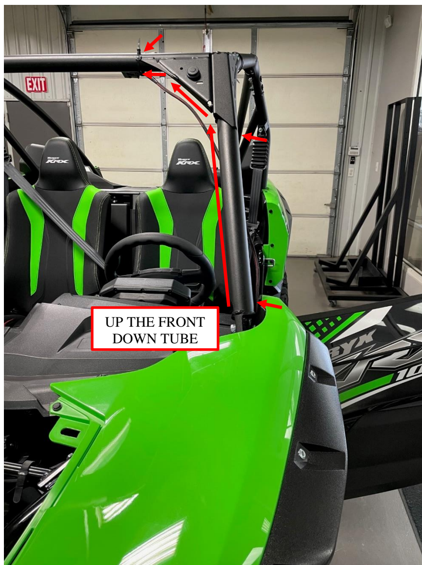
Figure 14: Chassis harness routing up driver's front down tube.
